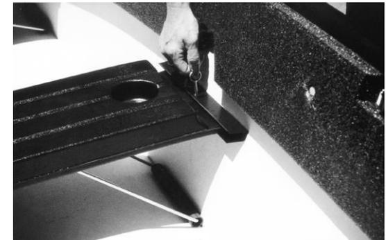
7. From outside boat, push the steel center seat support into center seam. If it is very tight, use the end of the boat opener to push into place while you lift the side of the boat, slightly. Do **NOT** do this when in the boat
