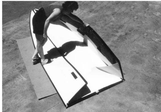
3. Place one end of the 2 STEP BOAT OPENER against the top tube of the OPPOSITE side from you. Place the curved hook cutout against the side of tube nearest to you. (See picture for approximate placement in the hull)
