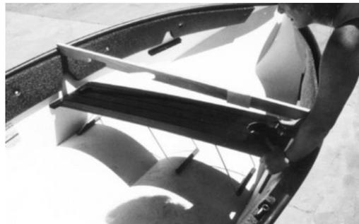
6. Line up hole at end of center seat with hole in seat bracket nearest you. Insert stainless steel locking pin as shown. Squeeze pin and twist as you turn. Now, insert pin in other side of seat. On 14' model install the other center seat the same way. On 8' model install front seat first.
