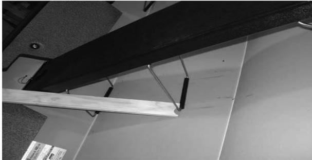
8. Each side of the transom is now ready to be swung out toward the rear of the hull just enough to allow installation of rear seat per sections 5 and 6. When you do this, lift both sections slightly so they rotate more easily.
