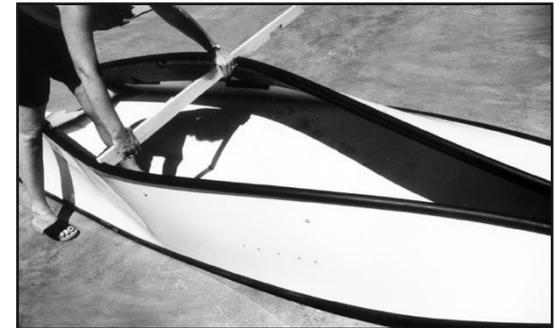
4. Use your leg to push away one side of hull until its far enough away to place other end of opener against the hull tube on opposite side. **IMPORTANT NOTE:** If necessary, insert the side seat support into a different hole under the seat so that they line up better at the bottom of the hull.
