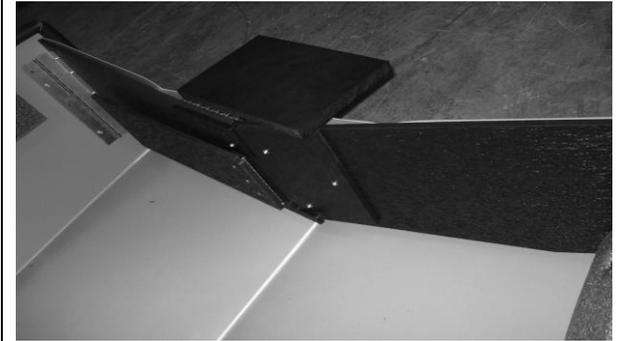
10. While making sure the transom halves interlock with each other, pull them all the way back. Swing transom support arm until it locks into the bracket at the edge of the rear seat.
