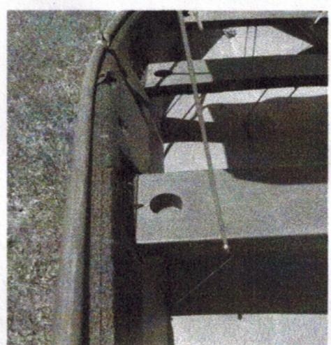
On a 12' boat, snap the shite strap to the front seat's outer, rear leg. (On other sized boats hook to the front leg of a seat.)
