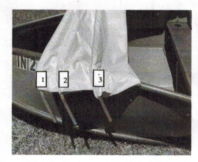
Open your boat insert and the Lay the seats. the canopy on bow of the boat as shown. Have the two closer curved tubes, #1 and #2, toward the front of the boat.
